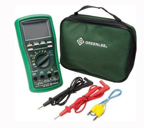
999 6758.8 © 2004 Greenlee Textron Inc. 12/04 Description The Greenlee DM-20 Digital Multimeter is a hand-held testing device with the following measurement capabilities: AC and DC voltage, DC current, and resistance. It also checks diodes, verifies continuity, and tests 1.5 V and 9 V batteries. Safety Safety is essential in the use and maintenance of Greenlee tools and equipment.
